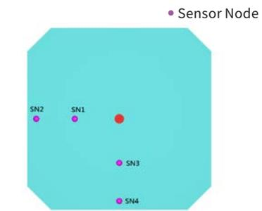
(c) Cavity geometry and pressure sensor location
